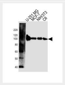
Western blot analysis of lysates from U251,MCF-7,mouse NIH/3T3,rat C6 cell line (from left to right), using VCP Antibody(Cat. #AW5229). AW5229 was diluted at 1:1000 at each lane. A goat anti-mouse IgG H&L(HRP) at 1:10000 dilution was used as the secondary antibody.
