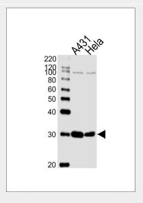
Western blot analysis of lysates from A431,Hela cell line (from left to right), using SFN Antibody (C-term)(Cat. #AW5163). AW5163 was diluted at 1:1000 at each lane. A goat anti-rabbit IgG H&L(HRP) at 1:10000 dilution was used as the secondary antibody.Lysates at 20ug per lane.
