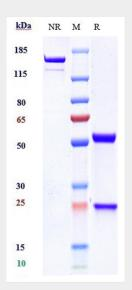
Anti-GPC3 / Glypican-3 Reference Antibody (Codrituzumab-MMAE) on SDS-PAGE under reducing (R) condition. The gel was stained with Coomassie Blue. The purity of the protein is greater than 90%
