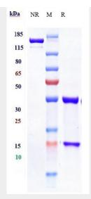
Anti-CTLA-8 / IL-17a Reference Antibody (vunakizumab) on SDS-PAGE under reducing (R) condition. The gel was stained with Coomassie Blue. The purity of the protein is greater than 95%
