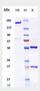
Anti-ERBB2 / HER2 / CD340 Reference Antibody (Trastuzumab duocarmazine) on SDS-PAGE under reducing (R) condition. The gel was stained with Coomassie Blue. The purity of the protein is greater than 95%
