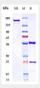
Anti-CD3 Reference Antibody (visilizumab) on SDS-PAGE under reducing (R) condition. The gel was stained with Coomassie Blue. The purity of the protein is greater than 90%
