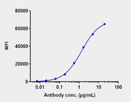
Raji cells were stained with Anti-CD20 Reference Antibody (rituximab) and negative control protein respectively, washed and then followed by PE and analyzed with FACS, EC87=1.334  $\mu$ g/mL
