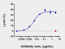
Anti-CD20 Reference Antibody (rituximab)-induced ADCC activity was evaluated using Raji Cell. The max Lysis rate was approximately 35%.
