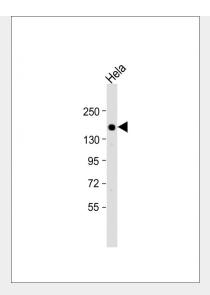
Anti-BRCA1 Antibody (N-term) at 1:1000 dilution + Hela whole cell lysate Lysates/proteins at 20  $\mu$ g per lane. Secondary Goat Anti-Rabbit IgG, (H+L), Peroxidase conjugated at 1/10000 dilution. Predicted band size : 208 kDa Blocking/Dilution buffer: 5% NFDM/TBST.
