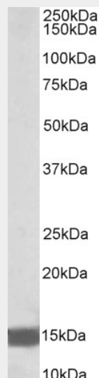
AF3834a (0.1 µg/ml) staining of Human Heart lysate (35 µg protein in RIPA buffer). Primary incubation was 1 hour. Detected by chemiluminescence.
