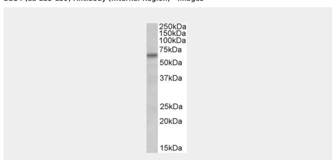
AF3424a (1  $\mu$ g/ml) staining of HeLa lysate (35  $\mu$ g protein in RIPA buffer). Primary incubation was 1 hour. Detected by chemiluminescence.
